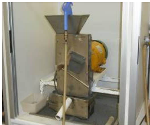
Figure 1. Soil preparation equipment and coarse grinder (<2 mm) used in this study. Fine textured soils can dry very hard and need to be disaggregated up using either a mallet or device such as a vice before coarse grinding.
