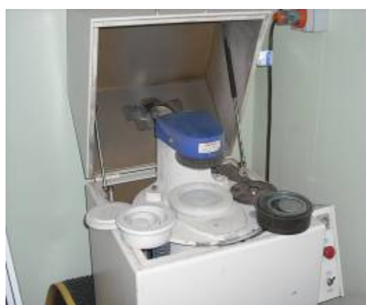
Figure 2. Soil grinding equipment used for fine grinding to <0.5 mm (left) or <0.05 mm using a ring mill grinder (right). Both fused zirconia rings and steel rings are shown.
