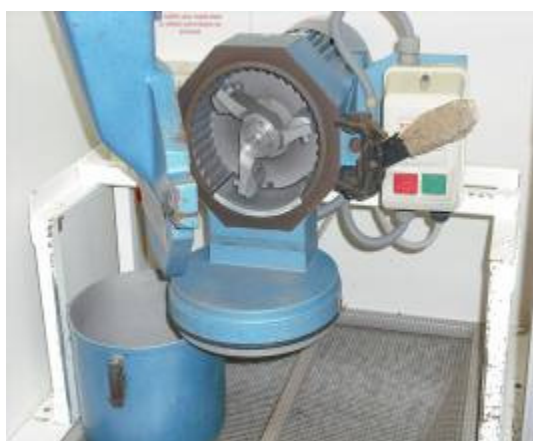
Figure 2. Soil grinding equipment used for fine grinding to <0.5 mm (left) or <0.05 mm using a ring mill grinder (right). Both fused zirconia rings and steel rings are shown.
