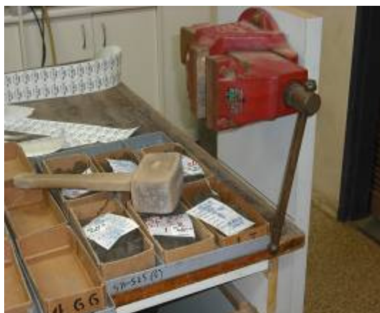
Figure 1. Soil preparation equipment and coarse grinder (<2 mm) used in this study. Fine textured soils can dry very hard and need to be disaggregated up using either a mallet or device such as a vice before coarse grinding.
